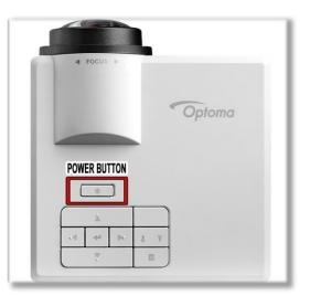
If the display in the glass seems to be offset or blurred, you can adjusts the projector focus by turning the focus ring left or right. If you need to adjust the position, quit the game into Windows and refer yourself with the grey bar all around the desktop wallpaper and the vertical center one.
